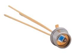
The SD 066-24-21-011 is a red enhanced Bi-Cell silicon photodiode used for nulling, centering, or measuring small positional changes packaged in a hermetic TO-46 metal package.
