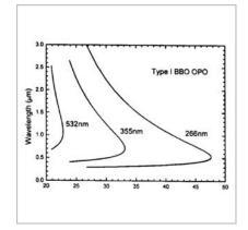
Figure 3: Type I OPO tuning curves of BBO
