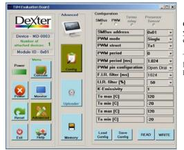
Clicking on the "Config" button allows you to change how the MD-0003 is configured to operate.
