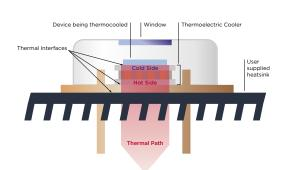
Figure 1 - Typical TO Style Package
