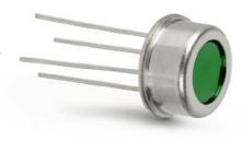
For pyroelectric detectors, the basic rule is that thinner chips provide higher detectivity. In this case, we use chips with a thickness of  $7\,\mu\text{m}$ . LTO chips are extremely robust and above all temperature stable. While other detector types in industrial environments require a Peltier element, LTO technology works well even at high temperatures without additional cooling.
