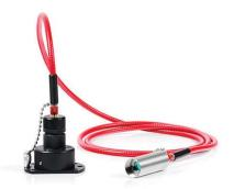
Output coupling collimators: in output coupling, the collimation of divergent light out of the connected fibre is important. The output coupling collimator, which is connected via an SMA connector, is used for this purpose. The optics used are adjustable along the z-axis and are available in three types of coatings from 350nm to 1600nm. To achieve different beam diameters, the output coupling collimators are available in various focal lengths.
