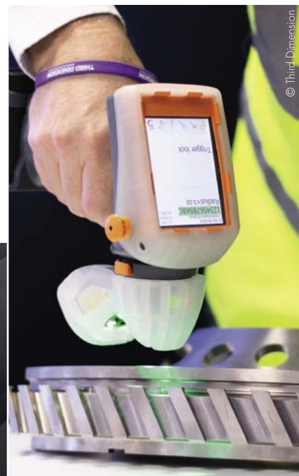
The portable gap measuring system GapGun with laser triangulation considerably reduces the working time and the costs of the manufacturing processes.
