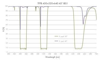
polarisers present a major challenge. The complex layer design is produced in our ion beam sputtering (IBS) facility, which enables particularly compact layer structures with good reflection properties.
