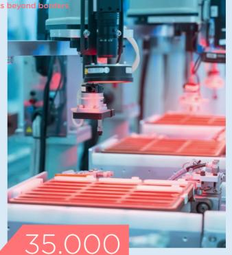
... 3D profiles can be captured by a machine vision system per second.
