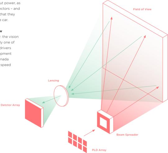
Flash LiDAR: with powerful emitters and highly sensitive detectors, LiDAR systems can be implemented without moving parts.
