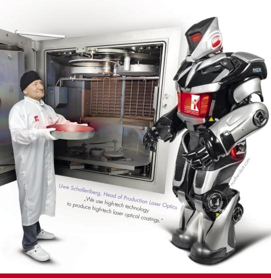
computer controlled. The layer thickness is permanently monitored and controlled during the entire process using an online monitoring system. This system makes it possible to achieve layer thicknesses with a precision of <0.5 nm.
