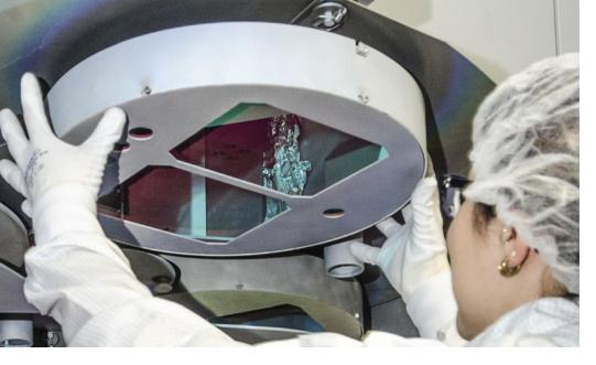
LASER COMPONENTS manufactures optics with diameters of up to 390 mm for these scientific institutions. To carry this out successfully, it is first necessary to select the right substrate and coating material.
